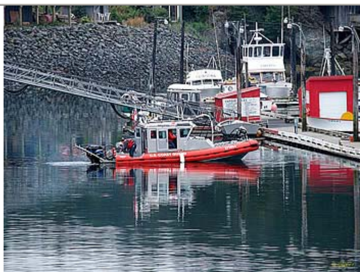
Spin her around and head for Homer. The SAFEBoat is 27 feet long and has two Merc 250's hanging off the stern.
